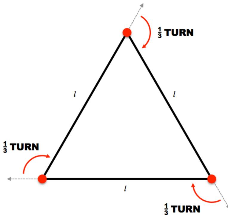
The sum of the exterior angles of the triangle must be 360 degrees, because the path begins and ends at the same position and orientation.
